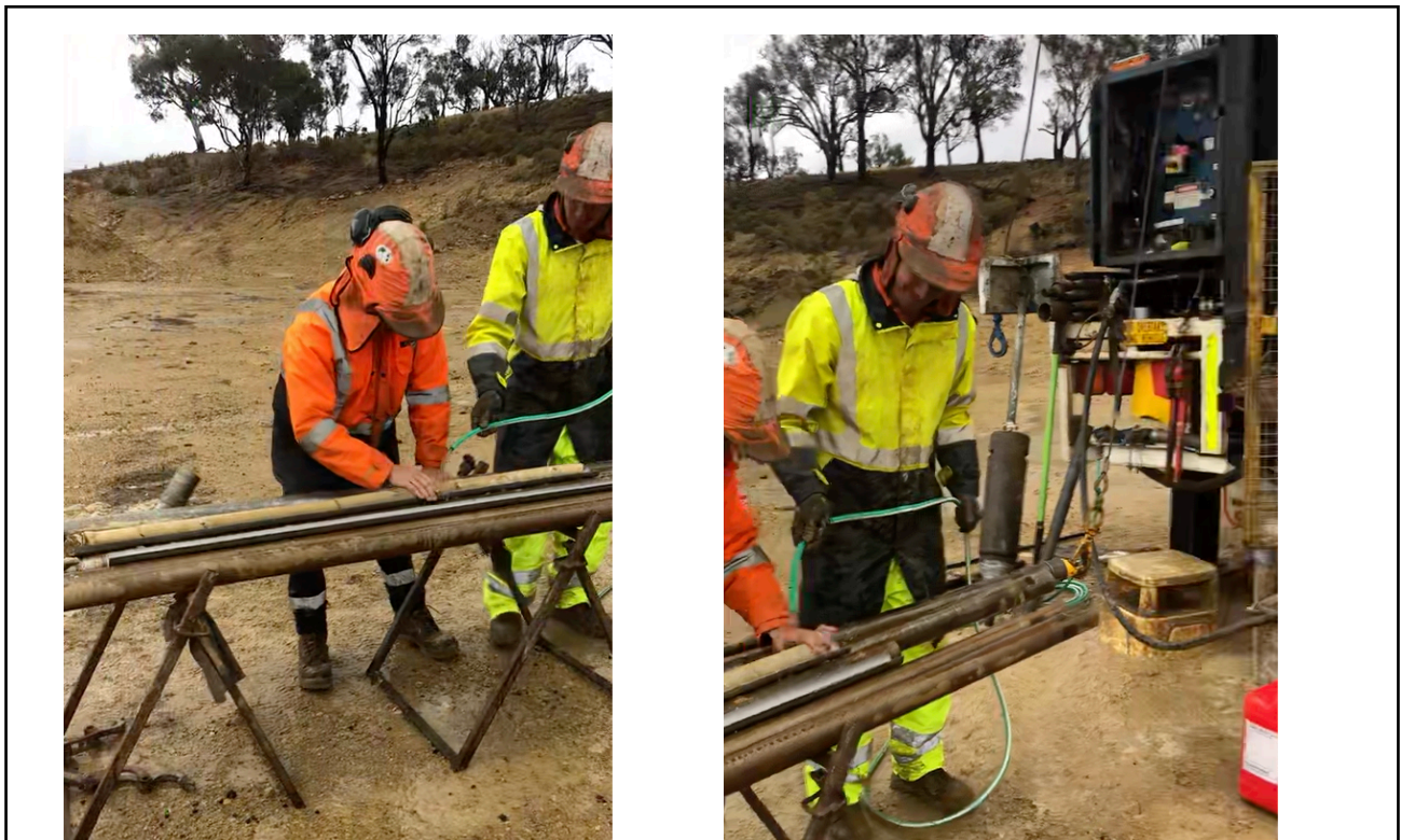
PHOTOGRAPHS 2.5 & 2.6: Core drilling by Douglas partners in and around the proposed quarry site reveals a quarry resource close to the ground surface
